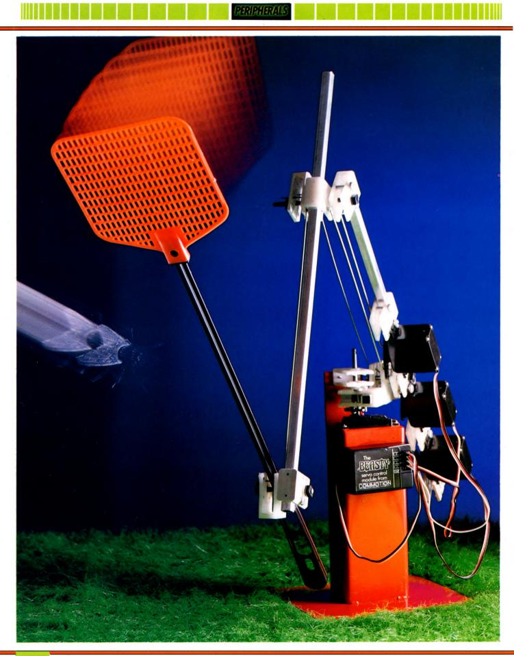
reasonably priced robots can be controlled from a home computer. They can see, read bar codes, draw, teach a high level programming language, and manipulate objects. There are two main categories of robots suitable for home micros—robotic arms, and floor turtles and buggies. These are supplied with 'user friendly' software, requiring no specific knowledge by the user.
